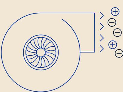
**1** Ionizers generate and disperse both negative and positive ions.
